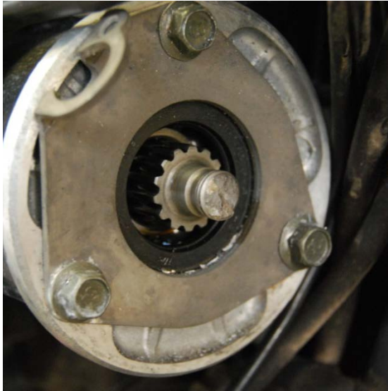
Picture 4. An inner thread must be tapped into the shaft. The engine does not need to be removed from the bike. Lift the bike so that the rear wheel can be removed. If possible, lift it somewhat higher, it will allow you to work more comfortably. Remove both footrests and the left exhaust. Remove the four hex bolts of the final drive. No need to remove the oil from the final drive. Remove the swing arm. You should now have free access to the middle drive shaft. Protect the bearing of the shaft by some cloth.
